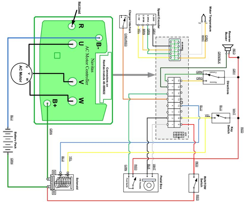
**Wiring Diagram – EZGO TXT 48 Conversion Kit**
