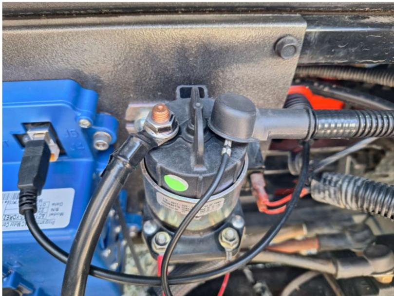
7. Connect the **AC ground wire** to the AC motor controller GND faston (next to the 3-pin connector) and route to the AC motor and use a motor mounting bolt to connect the AC ground wire.
