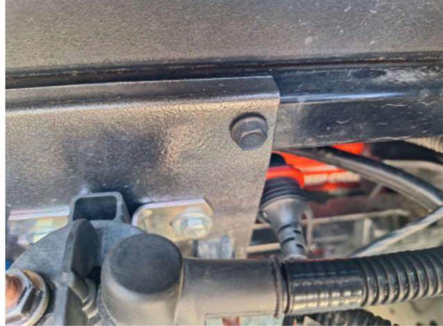
13. Install and connect the 3-phase motor wires as shown with U, V, W going to the correct terminals. U=BLK-TOP / V=RED-CENTER / W=WHT-BOTTOM. Torque bolts to specs on AC1 Manual **SPECIFICATIONS SECTION**. ZIP Tie the cable assembly using the OEM ring support shown above the motor.
