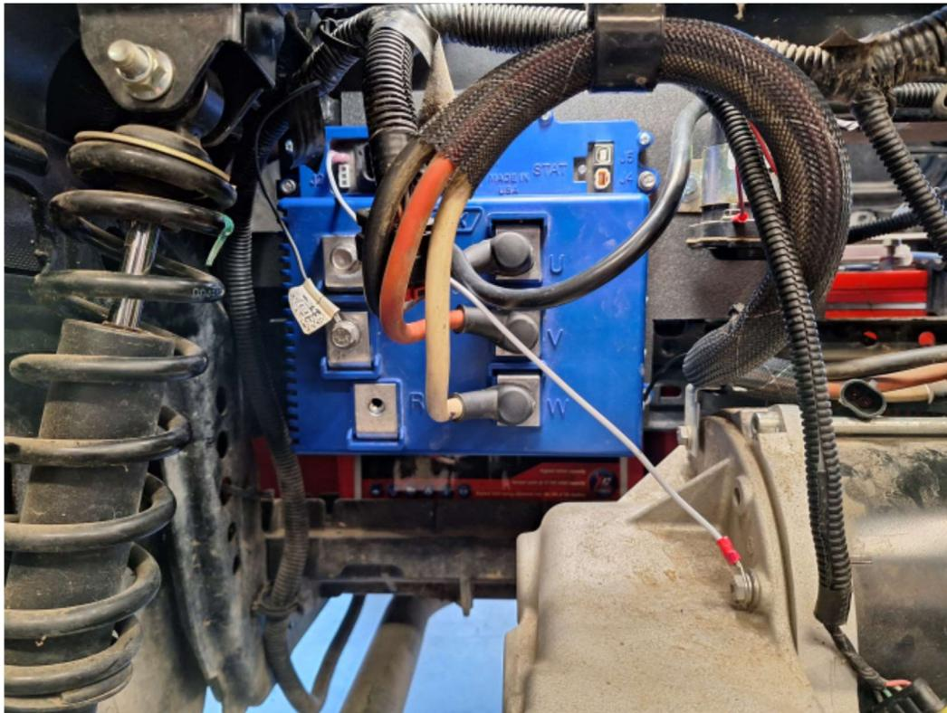
14. Insert the TOW/RUN switch with TOW on top, connect the wires removed earlier.
