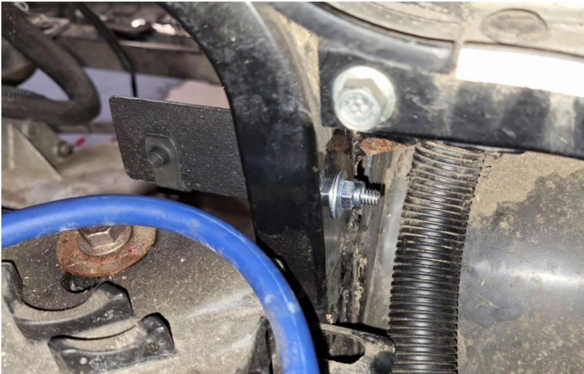
5. Mount AC1 Motor controller with CONNECTORS FACING UP towards the two mounting holes as shown.
