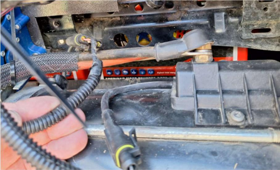
9. Install the proper ANN Fuse into the fuse holder. (See AC1 operators manual)
