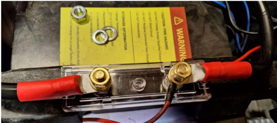
2. Connect cable 5/16" ring to the fuse, the 3/8" ring to the 400amp solenoid.
