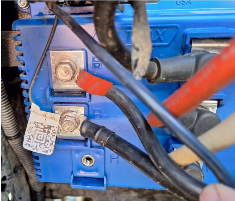
5. Connect the SOLENOID COIL wires as shown.
