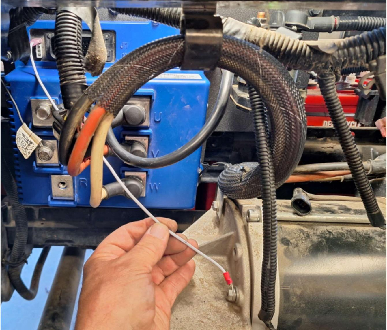
8. Connect the two sensor cables, the 4 pin speed sensor and 2 pin temp sensor.
