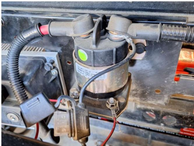
4. Remove wires and unplug wire harness, then remove the bolts holding the motor controller heatsink assembly. Remove from car:
