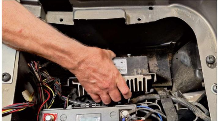
14. Remove the two wires from the resistor assembly. Replace with the supplied ORANGE and BLUE wires. They MUST BE MOUNTED AS SHOWN or the length will be wrong. (ORANGE on Left and BLUE on Right). The 5/16" Ring to the resistor, the 1/4" Ring to the Controller.
