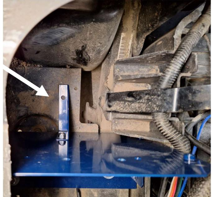
7. Locate the TWO 1/4-20x1" BUTTON HEAD CAP SCREWS to mount the resistor assembly. The DANAHER assembly will use the outside wider holes, the CURTIS assembly will use the inside smaller holes. Tighten with a 3/16" Allen wrench. Route the resistor wires between the car body and AC1 panel with Split loom protecting the wires.
