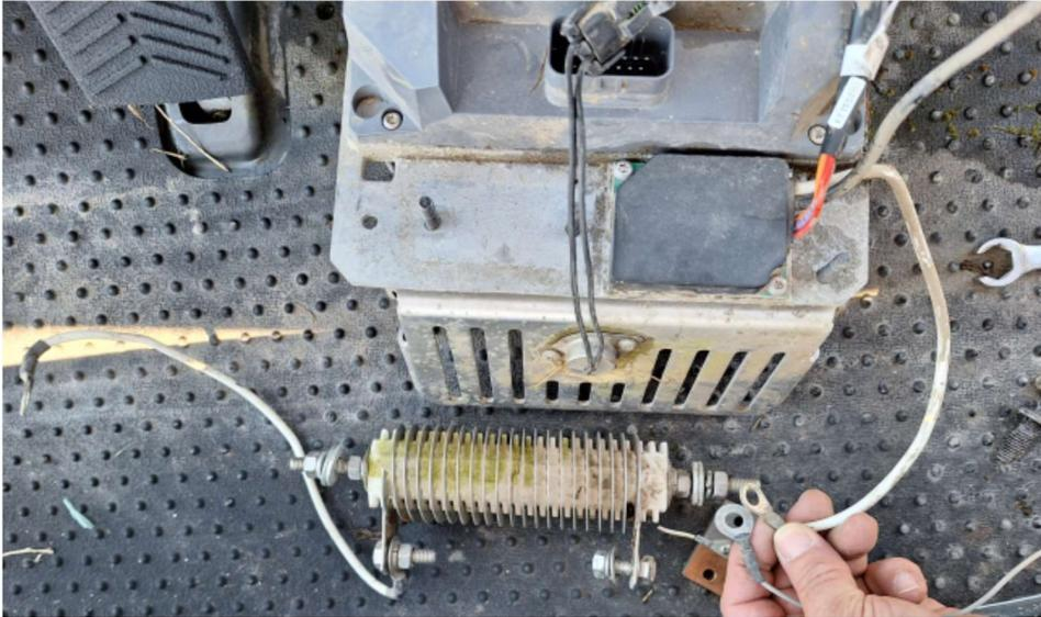
5. Prepare the resistor assembly for mounting on the new Alltrax AC1 Power Panel: The aluminum resistor assembly has two holes, we need to DRILL ONE HOLE to accommodate the 1/4-20 U-Spring Clip. Mark and drill 2.5" left of center and 5/8" up from bottom edge. Use a 19/64" or 5/16" drill bit.
