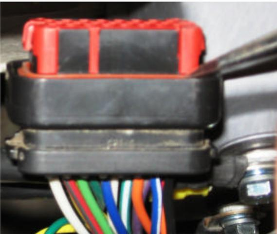
4. Now insert the <sup>Pin 11</sup> wire into Pin 17 as shown below.
